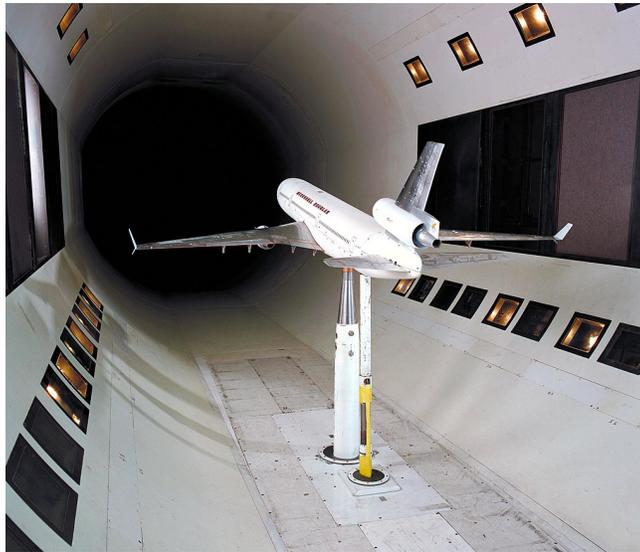
Figure 1.4: NASA wind tunnel with the scale model of an airplane (source: Wikimedia Commons, public domain)
