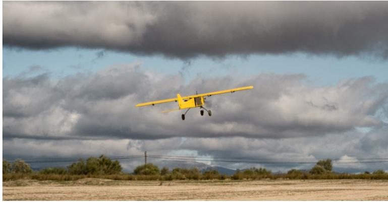
Figure 3.3: Small fixed-wing UAV used for framework evaluation.
